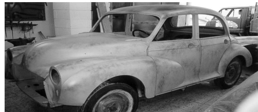
The body shell is primed and made ready for its first coat of green.
